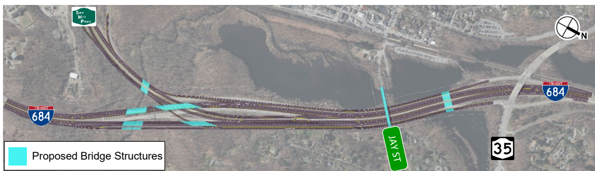
Figure FR-13: I-684 Interchanges 5 and 6 Full Reconstruction Concept
