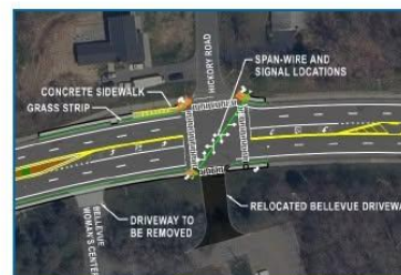
Proposed Traffic Signal at Hickory Road
